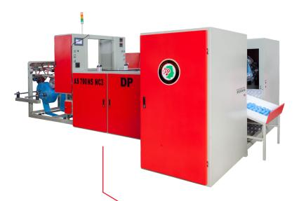
High speed bottom sealing machine with perforation and paper core rewind. Maximum speed up to 100 m/min.
